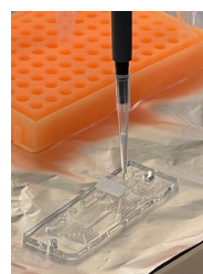
Mix the mashed lesion tissue with the reaction reagent and load it into the measuring chip.
