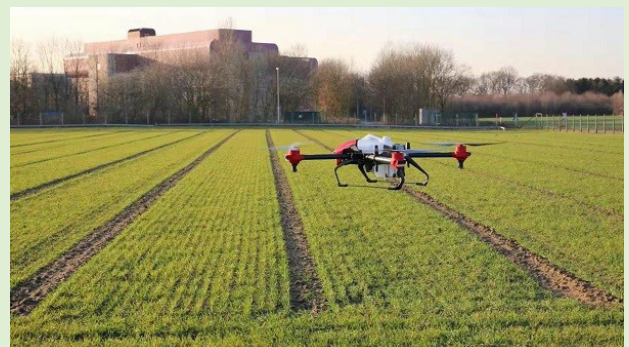
Drones (UAV) in agriculture production (pesticide application) is rapidly growing in popularity in Asia, for its outstanding advantages in efficiency, spray precision, and labor-savings.
